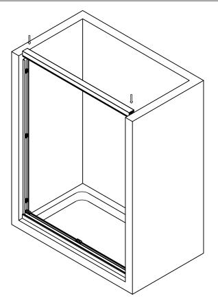
Step 7. Clip the top track onto the top of wall jambs.
