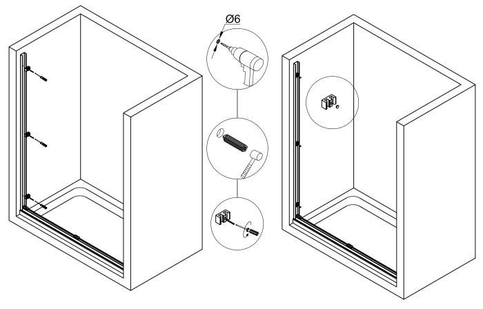
**Step 6.** Take wall jambs away, drill holes onto where marked on the wall, and put in wall plugs. Fix wall jambs to wall and glass stoppers onto wall jambs.
