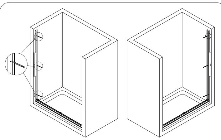
**Step 5.** Clip the two wall jambs onto each end of the bottom track. Adjust the wall jambs to make them 100% plumbing. Make holes positisions onto wall through holes on the wall jambs. See above drawings.
