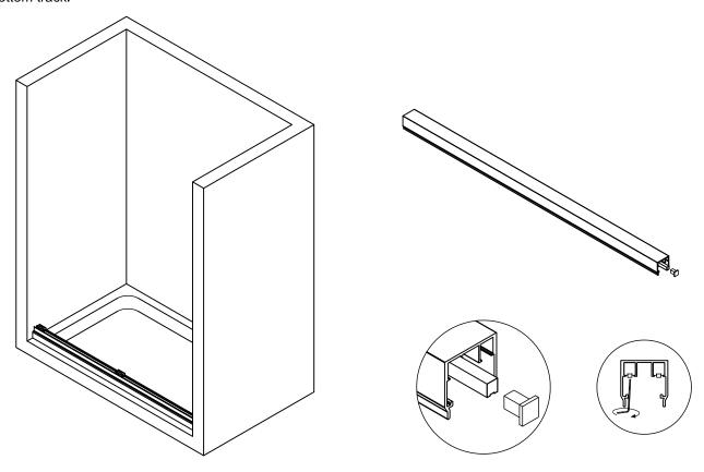
**Step 4.** Put the assembled bottom track to the installation position. Inset the soft closing dampers onto the top track using the soft closing locator to locate the position correctly. Fix them using a 2.5 Allen key. See above drawings.
