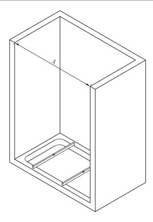
**Step 1**. Put the basin in the installation position adjust it to be 100% level.
