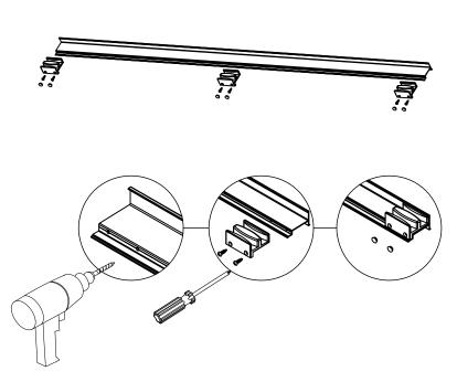
**Step 3.** Drill Ø3.2 holes onto the bottom track each end and the middle as above drawings. Fix bottom gliders onto the bottom track.
