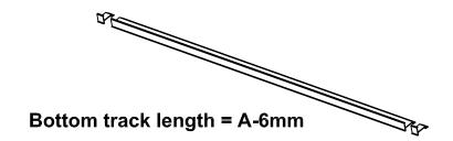
**Step 2**. Cut top and bottom track to be the correct length according to above instructions.
